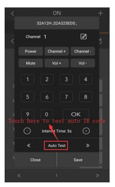
After adding the TV IR code into a room, we can find the corresponding TV in the category page. Touch the "TV" icon, we can go into the TV page. After that, we can control the TV via IR code.
