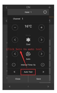
After adding the AC IR code into a room, we can find the corresponding AC in the category page. Touch the "AC" icon, we can go into the AC page. After that, we can control the AC via IR code.
