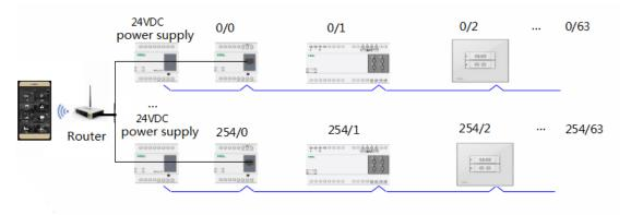
This is the basic method of controlling the HDL Buspro system by HDL ON, we can search and program the system devices by connecting the phone and the system in the same local area network (WIFI).
